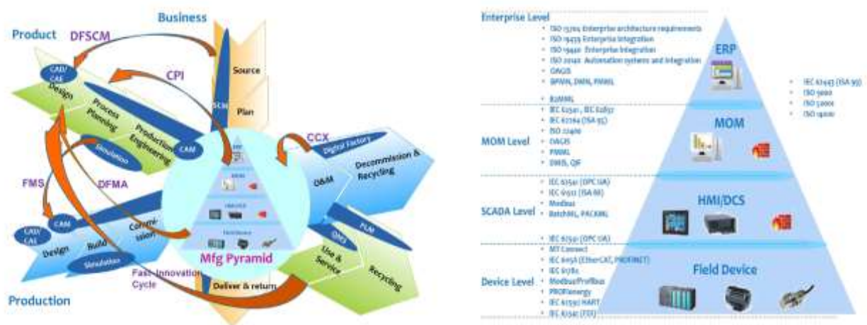
Figure 9: Smart Manufacturing Ecosystem aligned to IEC 62890 and ISA95 model.
