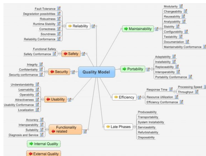
Figure 19 Model of system qualities according to ISO/IEC 25010 (not a complete list)
