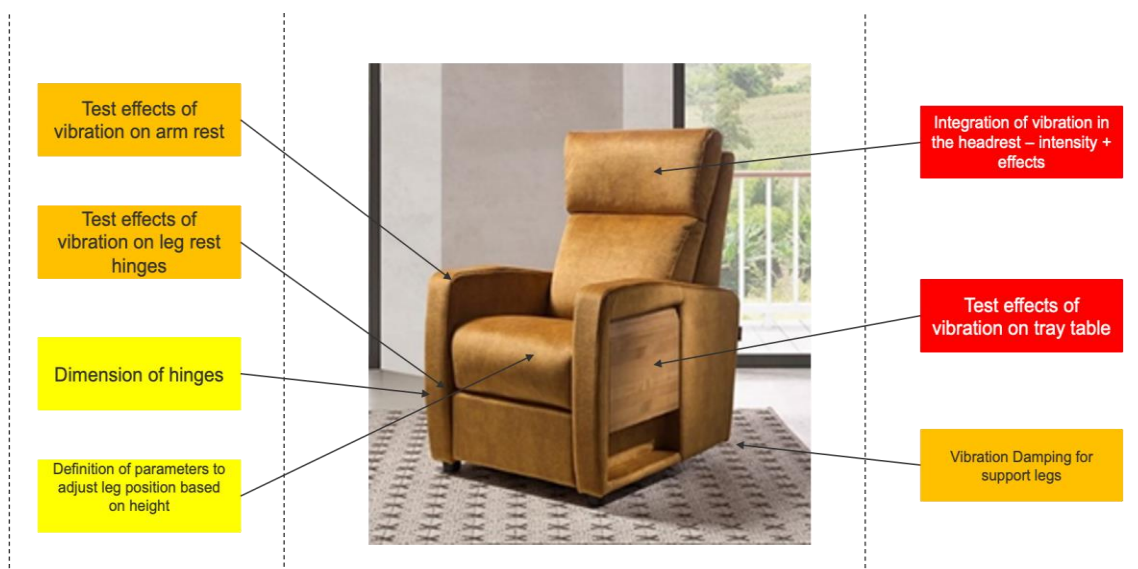
Figure 25. Mechatronic armchair technical requirement identification
