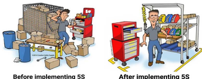
Figure 5. The objective of 5S is to make the workspace safe, efficient and effective
