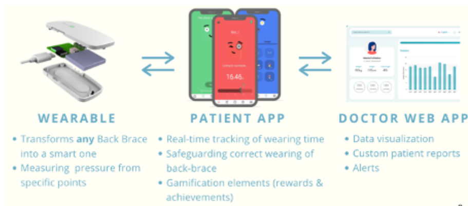
Figure 16: Connected patient and doctor web app to the IoT device
