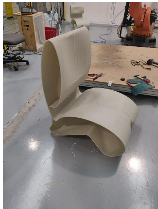
Figure 30. Prototype produced in Additive Manufacturing
